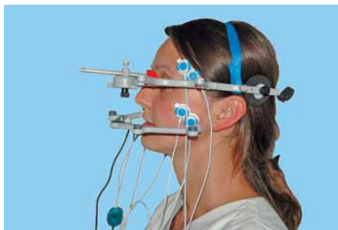
1 Experimental design. Snap-electrodes for sEMG of masseter and anterior temporalis muscles and ultrasound-based jaw-tracking system.
